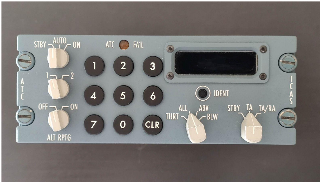
Front View of the ATC/TCAS Panel
